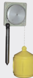
Beaded cable for tide measurements
